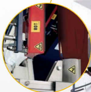
Teflon-coated sleeve-placket pressing device
